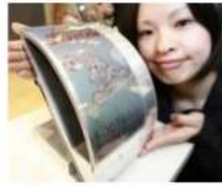
A Fujitsu employee displays the prototype model of an electronic paper display that is flexible and does not blur even if it is bent or pressed by a finger
